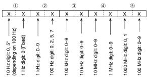
When the tuning step is selected 8.33 kHz (Air band), 100 Hz digit, 10 Hz digit and 1 Hz digit can be set 3 or 6.
