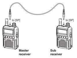
**NOTE: DO NOT** push any key on the sub-receiver during cloning. This will cause a cloning error.
