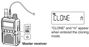
✓ CLONING MODE ENTRY (except Master receiver): When the CI-V baud rate (p. 56) is selected any other than "9600" or "AUTO," the following operations are required.
