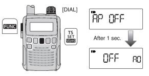
③While holding down [FUNC], rotate [DIAL] to select a desired time or to turn the function OFF.
