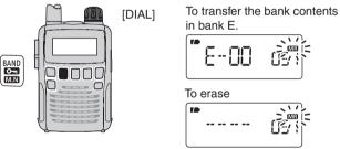
⑤ Rotate [DIAL] to select a desired bank channel.
