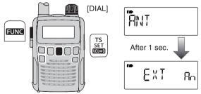
(5) While holding down [FUNC], rotate [DIAL] to select "BAR" when the Set mode has accessed from the AM broadcast band in AM mode; select "EAR" when the "ANT" item is selected for the strong signals.
