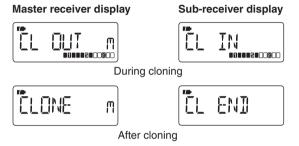
(4) When cloning is finished, turn power OFF, then ON to exit the cloning mode.
