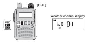
④ Push [BAND] to change frequency bands, or push [V/M] to select the memory mode.
